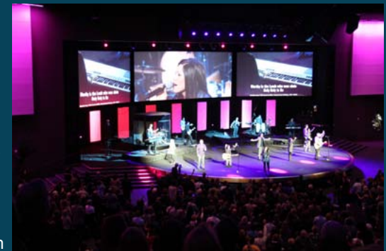
All three screens and projectors are on motorized hoists so they can be raised and lowered during the service without interrupting the video image.
