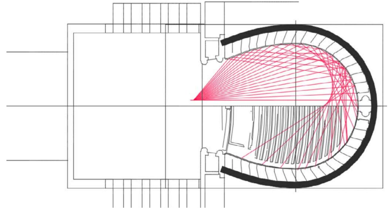
*Geometric acoustics study of an opera house falsely showing sound focusing.*
