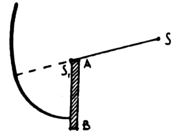
*Diffracted sound wave propagating from an edge (from Bagenal 3, p9)*
