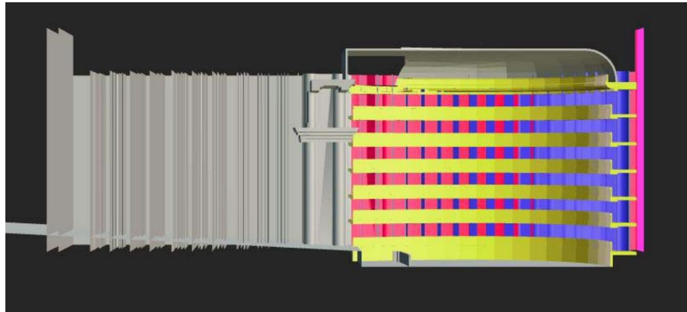
In contrast, the geometric acoustics model of the opera house – in this case La Scala – shows that the side walls (red) are largely screened from sound by the multiple balcony tiers, box dividers, and columns that form relatively small surfaces compared to the sound wavelengths of interest: [Interact with this image: https://p3d.in/MnzQf](https://p3d.in/MnzQf)
