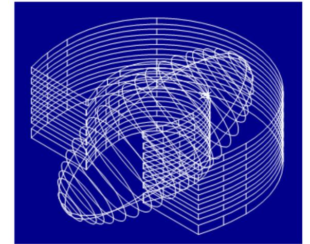
Intersection of ellipsoid at balcony fronts identifies the source locations of diffracted sound
