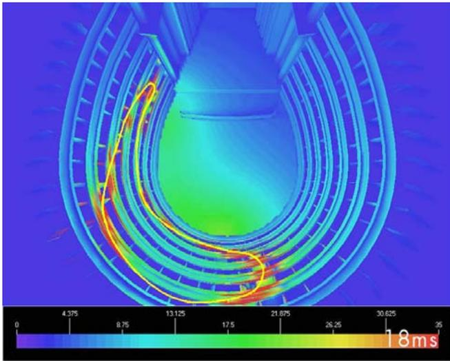
*The acoustic model is illuminated by light sources located at the intersection points (sketched here with a heavy line). This frame shows location of diffracted sound sources with 18ms delay. Watch the video.*
