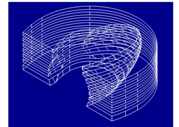
The solids subtracted to determine the locations of the Intersection of ellipsoid at balcony fronts
