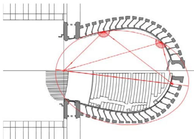
Ellipse representing the locus of an equal-delay-time contour. The foci of the ellipse are located at the source and the receiver. In 3D, this becomes an ellipsoid.
