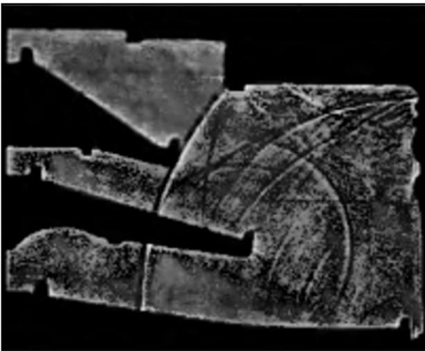
We have replicated Sabine's work using a digital wave-equation method, and this allows us to view wavefront propagation as a movie. As with Sabine's work, this method allows us to analyse a two-dimensional slice of the building.
