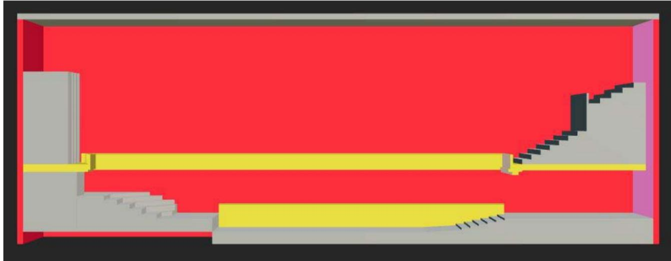
The objective acoustical characteristics of a concert hall (such as lateral, early, mid and late sound energy levels) can be modelled adequately with geometric acoustics studies because the side walls generally form large unbroken surfaces, shown in red in the model: [Interact with this image: https://p3d.in/fD7Dj](https://p3d.in/fD7Dj)
