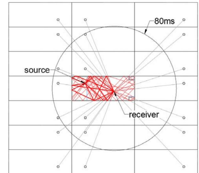
The objective acoustical characteristics of a concert hall (such as lateral, early, mid and late sound energy levels) can be modelled adequately with geometric acoustics studies because the side walls generally form large unbroken surfaces.
