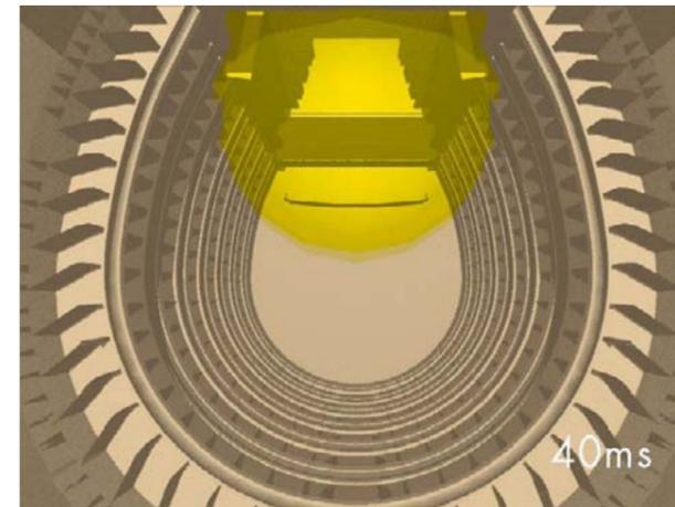
The direct sound propagating from the source, represented by a solid sphere. Diffracted sound will be generated where the surface of the sphere intersects the balcony fronts.
